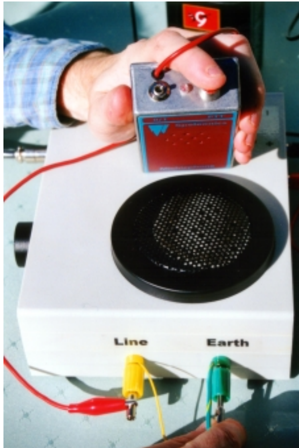
Testing a Michiephone handset using feedback and the Base Station.
